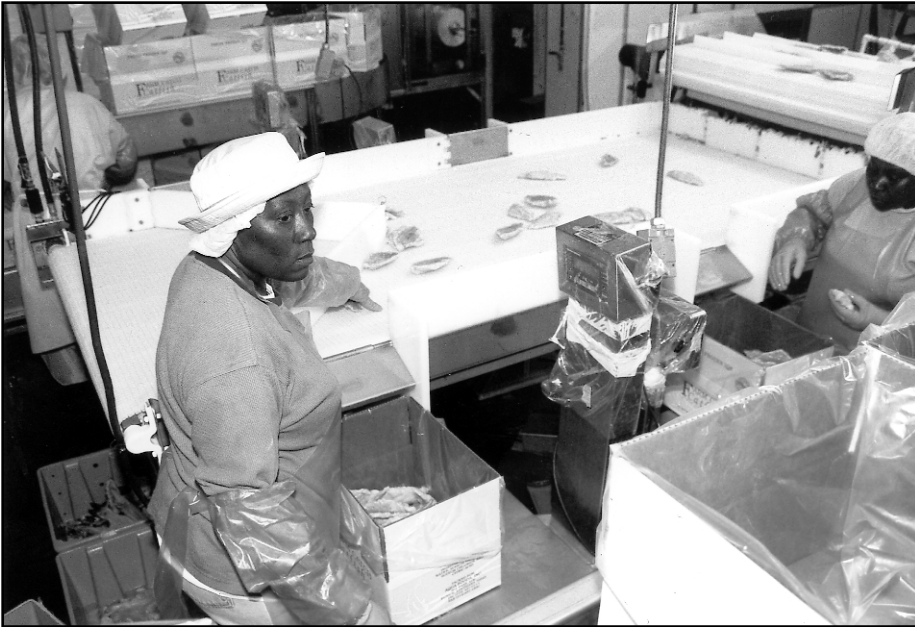
Figure 15. Frozen fillets are placed in plastic-lined boxes, weighed, and passed through a metal detector (if needed).
