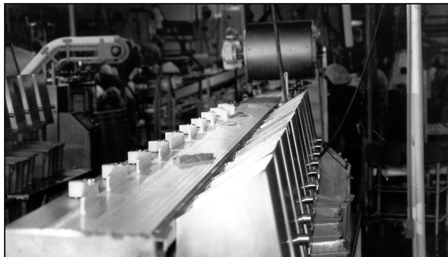
Figure 10. Automatic size graders used for dressed and filleted catfish.
