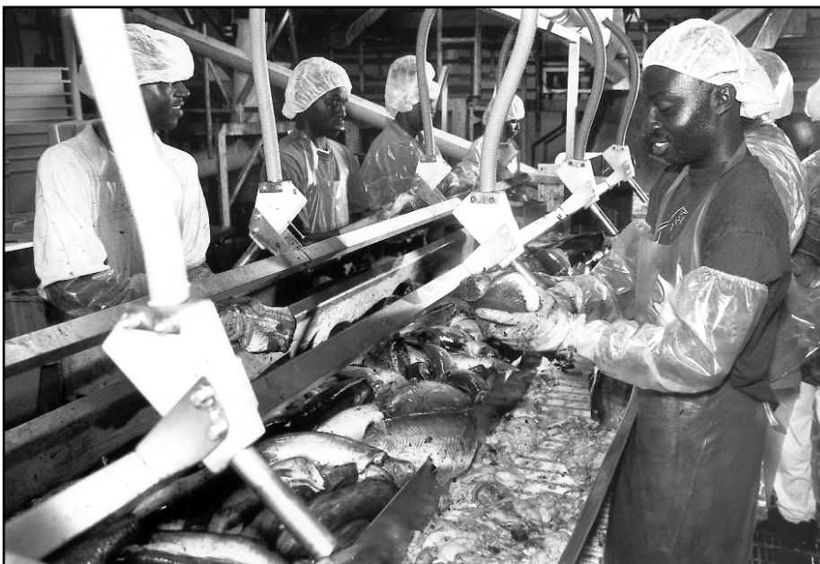
Figure 7. Evisceration (vacuum) stations to remove viscera manually before skinning.
