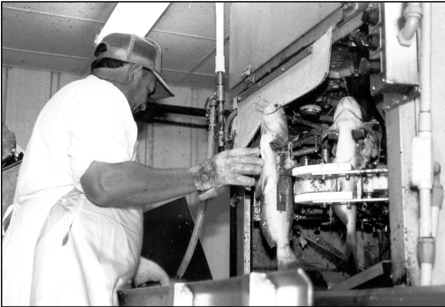
Figure 11. Automatic deheading station.
