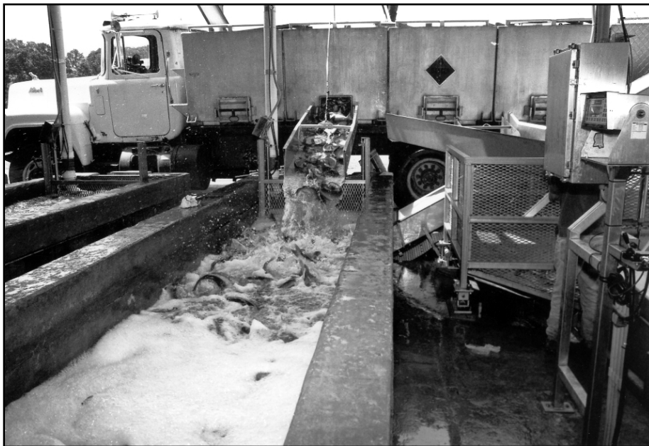
Figure 3. Fish are held in holding tanks (vats) before processing.
