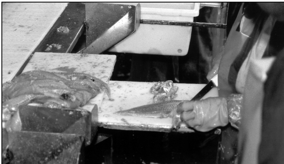
Figure 13. Manual trimming of fillets from automated lines.
